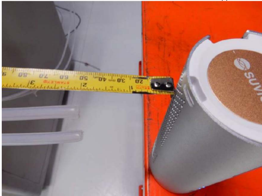
Located in the air stream 50 mm from the air outlet of the appliance
